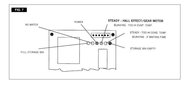
When the gear motor rotating speed is slowed below 1300 r.p.m. from the normal speed of 1400 r.p.m. the Electromagnetic Safety Device transmits an electrical signal to the MICROPROCESSOR to **stop immediately** the unit operations like it occures for the wrong rotation, with the lighting-up of the 3RD YELLOW WARNING LED. This to relieve from the excessive load all the electrical and mechanical components of the entire Drive System and extend their durability.
