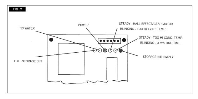
**NOTE**. If, after ten minutes from the compressor start-up, the evaporating temperature has not dropped down to a value lower than -1°C (30°F) the evaporating temperature sensor detects such an abnormal situation and stops consequently the unit operation.
