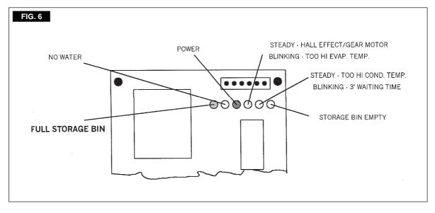
NOTE. The ICE LEVEL CONTROL (INFRA-RED SYSTEM) is independent of the temperature however, the reliability of its detection can be affected by dirt and scale sediment which may deposit directly on the light source and on the receiver.
