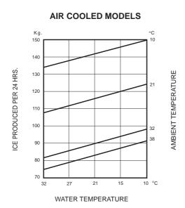
**NOTE**. The daily ice-making capacity is directly related to the condenser air inlet temperature, water temperature and age of the machine.
