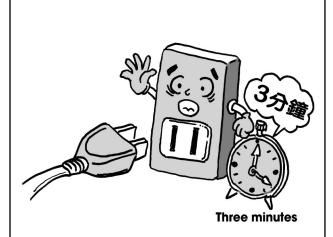
短時間間隔拔掉電源,會造成保險絲或斷路器跳脫。 Pull out the plug at short intervals would cause broken fuse and the circuit breaker off.
