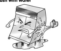
易產生漏電之原因。 This would cause an earth leakage.
