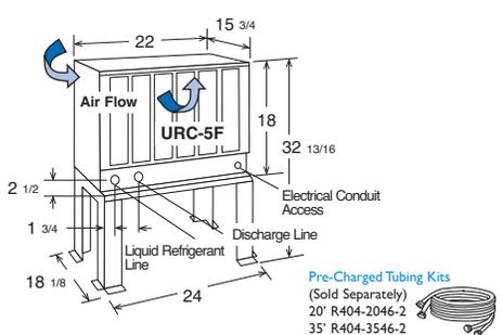
Voltage supply for the URC Remote Condenser is supplied from the Ice Maker.
