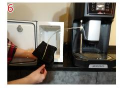
Clean tube and hose with clean wet towel. Place milk back in refrigerator. Press Enter to finish cleaning.
