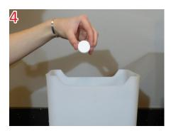
Dissolve an Egro Milk System Cleaning Tablet in a container with warm water. Place into refrigerator and press Enter.
