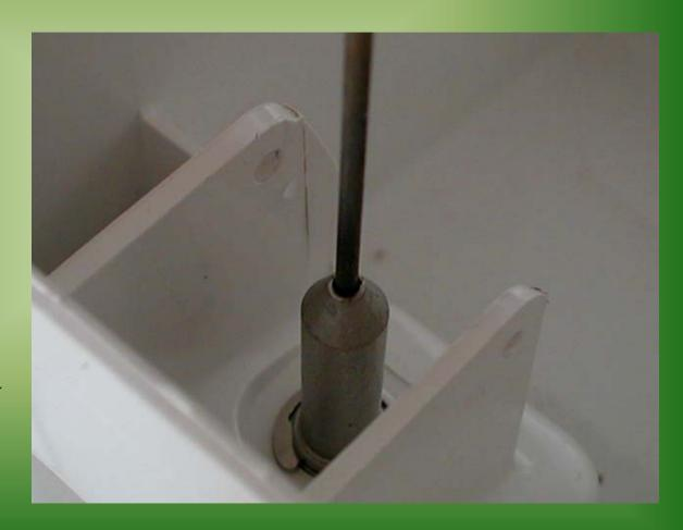
In case of water into the water reservoir check for any scale deposit onto the two metal pins of the water level sensor.....
