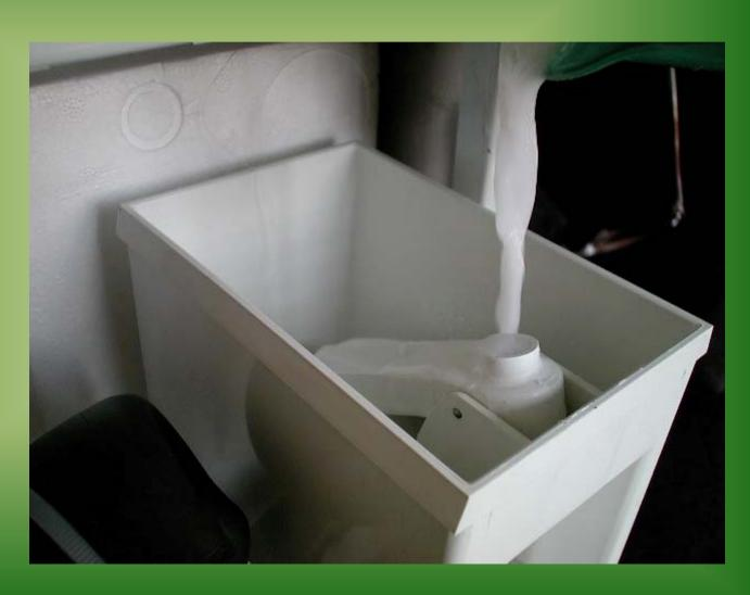
Once empty the bucket open the water tap so to allow new fresh water into the water reservoir and leave the machine running for approximately 10 minutes.
