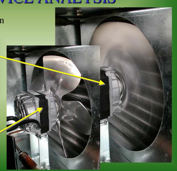
In case the power during the OFF mode is between 140 and 170 V the fan motor is keeping running but at lower speed that can cause an overheat of the same.
