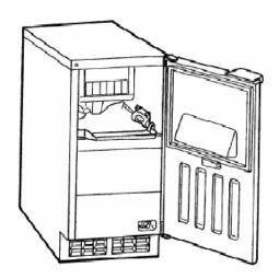
The AM-50 door can be field converted from the standard right hinged door to a left hinged door without the use of any additional hinge kits. The AM-100 and AM-150 use a spring loaded drop down door design therefore can not be reversed.
