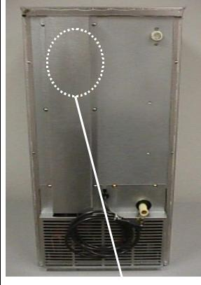
The AM series uses a thermostatic bin control located on the right rear side of the ice storage compartment. This control will open when ice touches the sensing bulb and the unit will shut down
