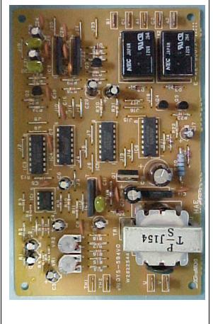
The AM series uses a combination thermistor and control board to control the sequence of operation. When the toggle switch is placed in the "ON" position and the bin control calls for ice, the unit will begin in the initial harvest cycle. Starting the unit in harvest allows the compressor to start in an unloaded condition, greatly extending the life of the compressor. This operation is common among all Hoshizaki cube icemakers.
