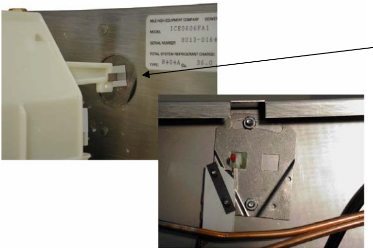
Proper position of wire bale switch actuator
